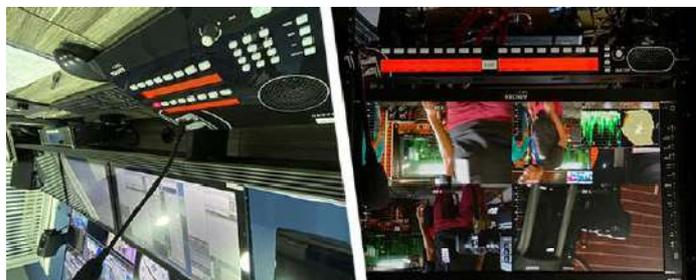
Also, for the Vision operators TP8116 panels were installed for communications and KROMA by AEQ Series LM8018 serves as shading monitors. These monitors are featuring SFP modules for fiber link IP SMPTE 2022 video.
