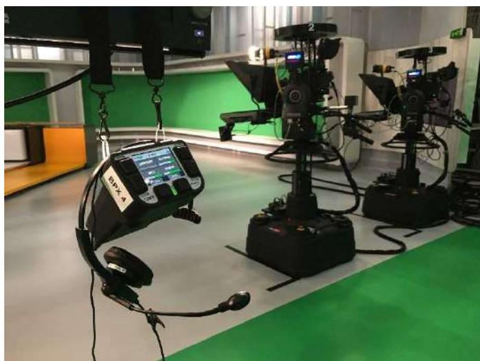
Xplorer is more than a belt-pack: it is a true wireless user intercom panel. Based on Wi-Fi technology, it features a user interface with 4 shortcut keys organized in pages, another two programmable keys and a multifunction screen.
