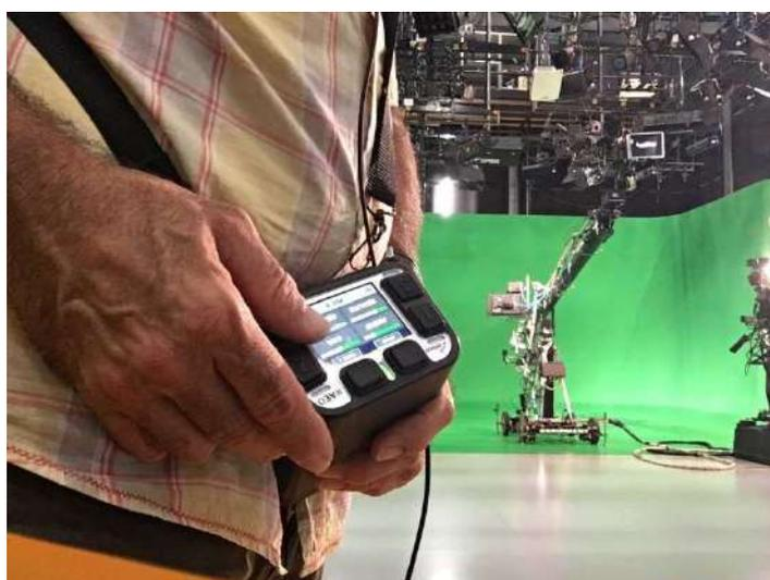
XPLOER beltpack has dual volume control in order to quickly adjust the level of the main peer, differentiating it from the rest.
