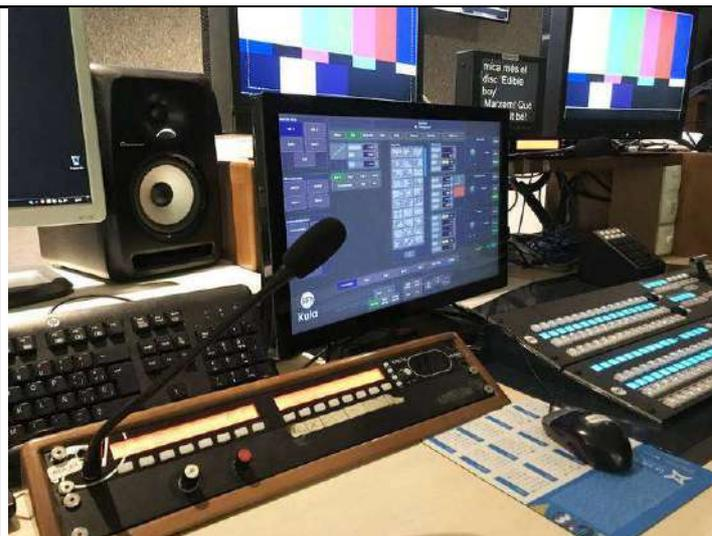
Series-8000 user panels have been designed to achieve a high, broadcast-compliant, audio quality level allowed by CONEXIA and digital technology. Audio is digitized and processed with 24 bits at 48 kHz, providing full 20Hz to 20 kHz audio bandwidth and much reduced noise and distortion levels. Ease of installation has also been kept in mind, that's why a redundant IP port, managing audio in the international DANTE-AES67 high-quality format, is included.
